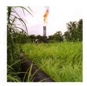
Everywhere close to the oil-wells so called metcheros – matches – can be found. They are burning associated gas, a side product of oil drilling. The constantly burning torches are causing great heat in their surrounding – killing thousands of insects seeking light – and are bringing about high air pollution with severe health effects for the people living in their neighborhood, like headaches, respiratory problems and cancer.
